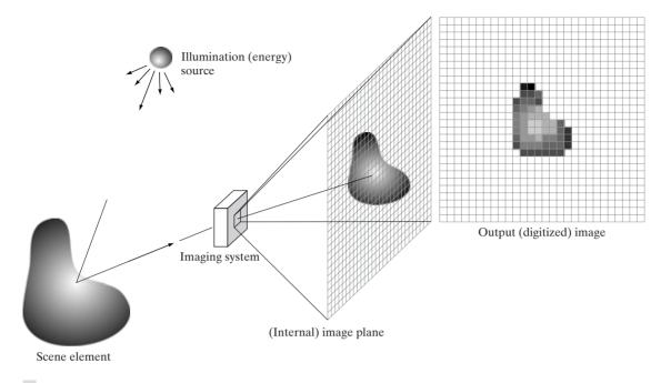
**FIGURE 2.15** An example of the digital image acquisition process. (a) Energy ("illumination") source. (b) An element of a scene. (c) Imaging system. (d) Projection of the scene onto the image plane. (e) Digitized image.
