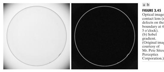
**FIGURE 3.45** Optical image of contact lens (note defects on the boundary at 4 and 5 o'clock). (b) Sobel gradient. (Original image courtesy of Mr. Pete Sites, Perceptics
