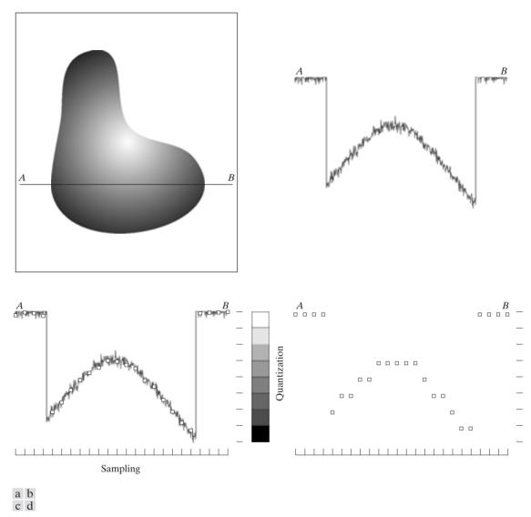
**FIGURE 2.16** Generating a digital image. (a) Continuous image. (b) A scan line from A to B in the continuous image, used to illustrate the concepts of sampling and quantization. (c) Sampling and quantization. (d) Digital scan line.
