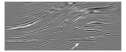
Seismic interpreters look for these "bright spots" to find oil and gas. The layers above also are bright, but their brightness does not vary as strongly across the layers. Many seismic reconstruction algorithms have difficulty imaging this target because of the faults above it.
