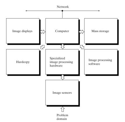
FIGURE 1.24 Components of a general-purpose image processing system.
