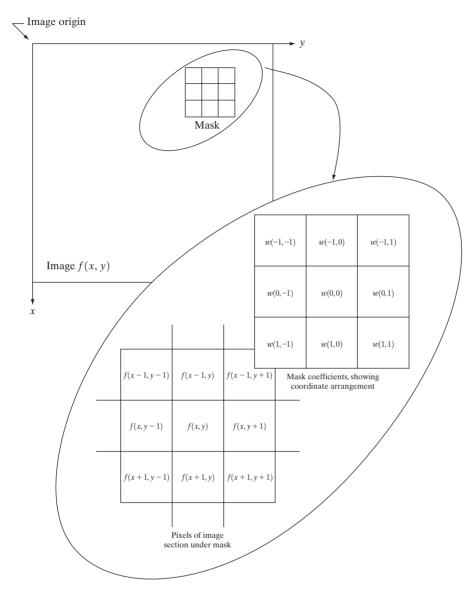
**FIGURE 3.32** The mechanics of spatial filtering. The magnified drawing shows a  $3 \times 3$  mask and the image section directly under it; the image section is shown displaced out from under the mask for ease of readability.
